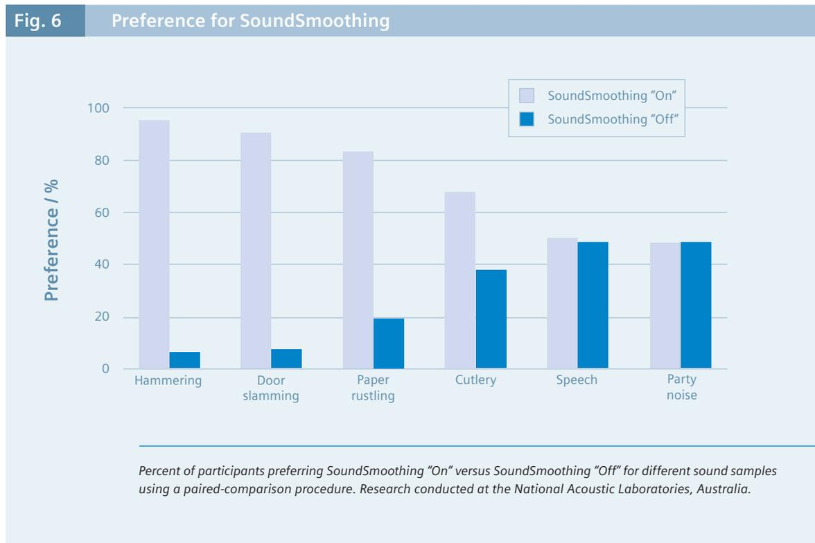
As discussed in the preceding section, the new SoundSmoothing algorithm introduced by Siemens in CENTRA has the potential to reduce the impact of transient environmental signals, and thereby provides a more pleasant listening experience. It was important, therefore, to conduct behavioral research with SoundSmoothing to determine, if the proven laboratory advantages also were considered a significant improvement by actual hearing instrument wearers.
